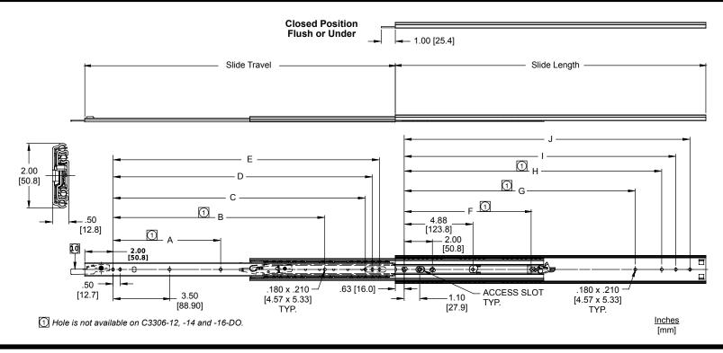
Finish: Bright electro-zinc (C) plating only Mounting: Bracket or hard mounting
